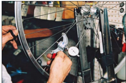
Measuring spoke tension with tensiometer
